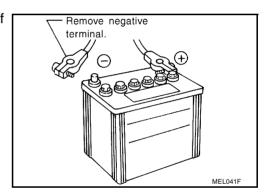
Check the charge condition of the battery.
