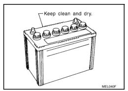
When the vehicle is not going to be used over a long period of time, disconnect the negative battery cable.
