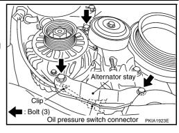
11. Remove alternator assembly to the direction of under side the vehicle.
