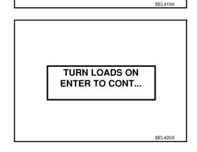
10. Raise and hold the engine speed at 1,500 to 2,000 rpm for about 5 seconds, then return the engine to idle. Once the increase in engine rpm is detected, press "ENTER" to continue.
