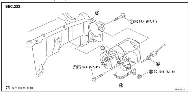
1. Starter motor mounting bolt
