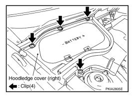
2. Disconnect negative battery cable and positive battery cable.
